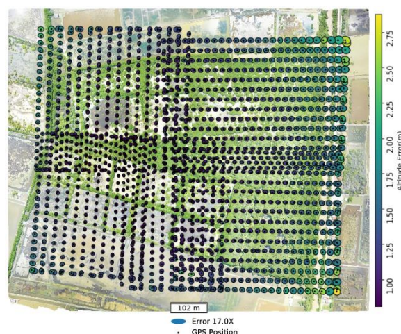
Figure 4. RMSE Orthophoto Imagery at Dimension Z (altitude)
