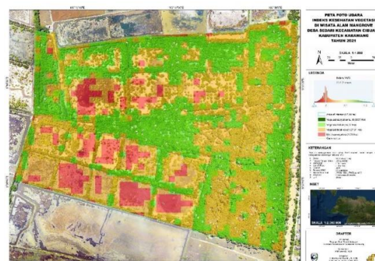
Figure 5. Aerial photo map of mangrove health index with application of VARI algorithm
